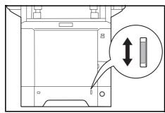
There is a paper gauge on the right side of the front of the paper cassette to indicate the remaining paper supply. When paper is exhausted, the pointer will go down to the level of (empty).
